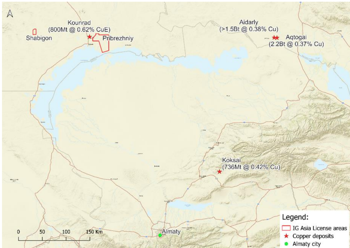
Figure 4: Large Porphyry copper \pm Mo/Au systems in South Central Kazakhstan
